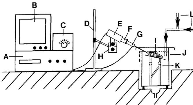
**Fig. 1.** Instruments and equipment used for bivalve endoscopy. (A) Video cassette recorder, (B) video monitor, (C) halogen light source (150 W), (D) support stand, (E) CCD video camera, (F) zoom lens, (G) endoscope, (H) micromanipulator, (I) bivalve, (J) plastic bucket with lid, (K) adjustable holding stand, (L) seawater and particle inflow
